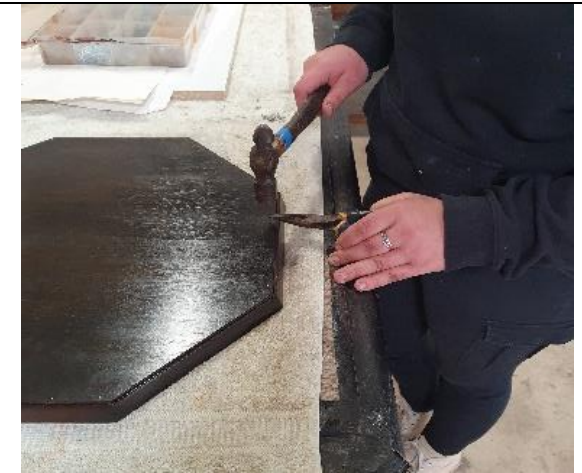
Photograph 68: Nailing on backboard.
